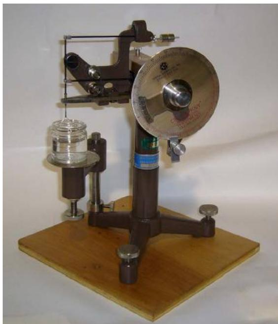
Figure 47 A real view picture of the CSC-DuNouy tensiometer used to measure oil-water interfacial tension (Courtesy of Francois Ayello).
