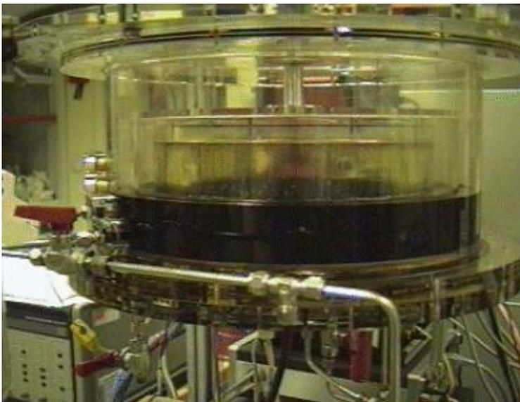
Figure 7 Small scale apparatus, carousel, used for studies of water entrainment and breakout in crude oil (Pots *et al.*, 2006).
